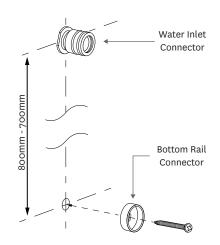
Screw the bottom rail connector to a wall stud making sure it is vertically in line with the top rail connector. Maximum centre distance between the top and bottom shower connections is 800mm.
