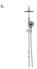
Make sure a washer is in both ends of the hose. Screw hose onto lower outlet on wet rail, attach handset and place firmly in holder. Tilt and rotate head to the desired position.
