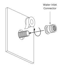
Loosen the 2 grub screws with the Allen Key supplied and remove Water Inlet Connector from diverter. Apply thread tape (or Similar) to the  $\frac{1}{2}$ " connection and screw Water Inlet Connector onto the  $\frac{1}{2}$ " connector.
