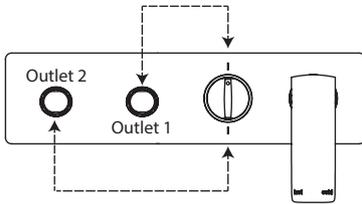
Both hand shower and bath outlet can be installed to either outlet 1 or outlet 2.
