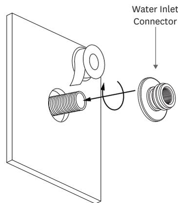
Loosen the 2 grub screws with the Allen Key supplied and remove Water Inlet Connector from diverter. Apply thread tape (or Similar) to the ½" connection and screw Water Inlet Connector onto the ½" connector.
