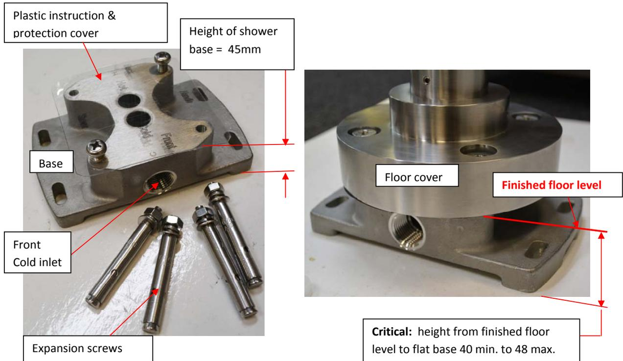
1. Position base following orientation on plastic instruction cover fitted to base. Locate front/cold and back/Hot allowing sufficient room around base for water connection
