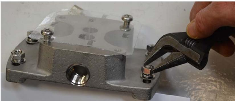
3. Ensure height to finished floor level from base (40mm min to 48mm max.) is considered so floor cover will sit down on finished floor level
