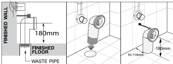
Insert waste pipe into floor at a setout of 95-110mm and 180mm above finished floor and fix bracket into position as per diagram above.
