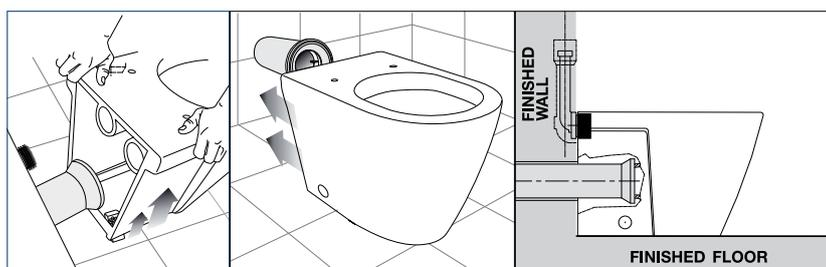
Push pan back into position. Ensure that you make a firm connection with inlet and outlet pipes and avoid disturbing the floor fixing brackets. Flush test for leaks.
