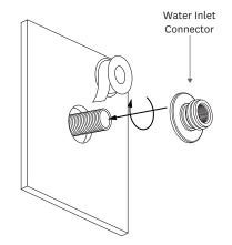
Loosen the 2 grub screws with the Allen Key supplied and remove Water Inlet Connector from diverter. Apply thread tape (or Similar) to the  $\frac{1}{2}$ " connection and screw Water Inlet Connector onto the  $\frac{1}{2}$ " connector.
