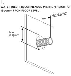
Install a <sup>1</sup>/<sub>2</sub>" male threaded connection at the recommended height on wall, ensuring that a minimum of 13±2mm of thread protrudes past the finished wall.
