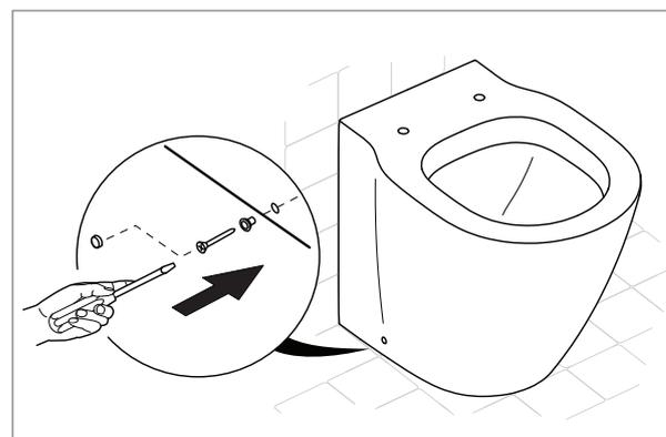
The installation of the toilet suite shall be in accordance with AS/NZS 3500
