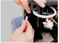
Run the the brine hose from the inside though the bore to the outside and insert it as far as it will go (a depth of about 15 mm) in the connection angle.
