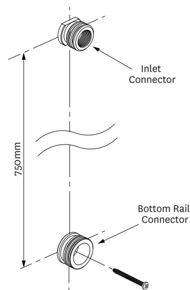
Screw the bottom rail connector to a wall stud vertically in line with the inlet connector and at the correct distance.
