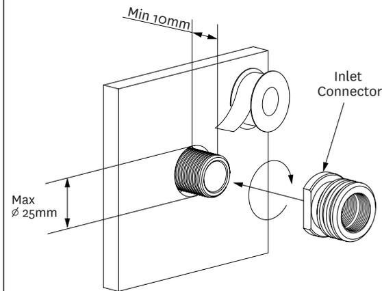
Install a 1/2" male threaded connection at the recommended height on wall, ensuring that a minimum of 10mm of thread protrudes past the finished wall. Apply plumbing tape (or similar) to the 1/2" threaded connection, then screw the inlet connector onto it.
