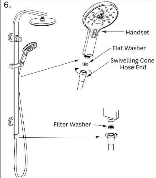
Make sure a washer is in both ends of the shower hose. Screw one end of the hose to the bottom of the shower rail, attach handset and place firmly in holder.
