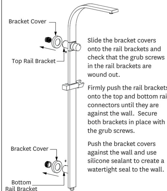
Slide the bracket covers onto the rail brackets and check that the grub screws in the rail brackets are wound out.
