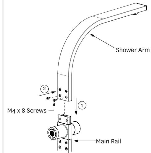
Assemble the shower arm by sliding it onto the top end of the main rail. Secure the shower arm in place with the screws provided.
