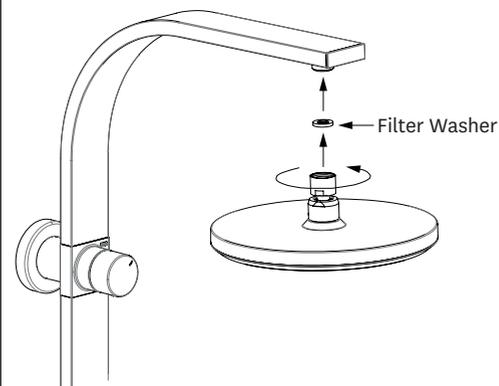
Remove the protective cap from the shower head ball joint and screw the shower head onto the shower arm, ensuring that the filter washer is in place.
